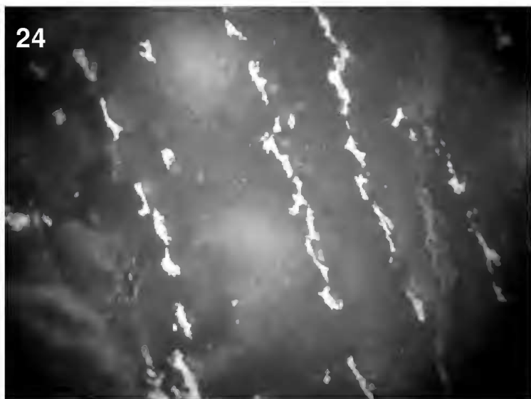
Fig.24- Concomitant reflected and transmitted light photomicrography. Metal-sulfide melt drops and troilite along plane fractures in olivine. Length of field 0.2mm.
